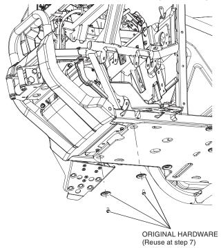
3. Install the mount plate on the vehicle using two 14  $\times$  30 mm hex flange bolts and two 14 mm hex flange nylon nuts (not shown). Hand tighten.
