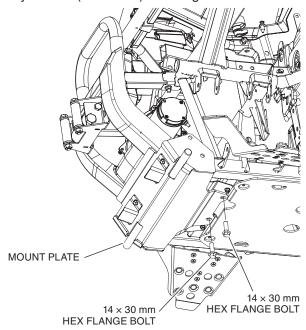
4. Install one  $14 \times 45$  mm hex flange bolt into the existing weld nut on each side of the CBU frame.
