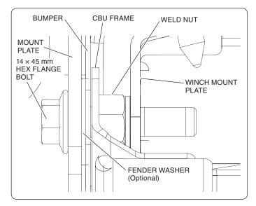
5. While holding the mount plate up against the bumper and frame, tighten the bolts to the values specified in the TORQUE CHART.
