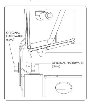
2. Remove the two front screws of the plastic skid plate.
